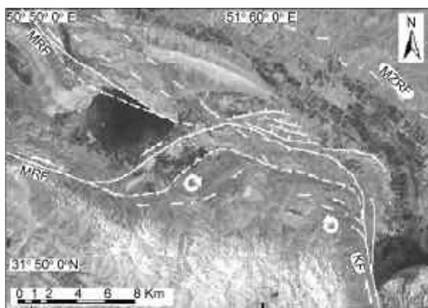
Figure 4. Step over made by two left-stepping strike-slip faults of Kazerun fault from south and MRF from NW makes a pop-up structure in their connection point. Elevated young materials in front of structure gave rise to local sliding and gravitational collapses and were reflected as normal faults on the map, see Figure (5) for location.
