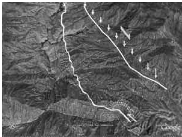
Figure 13. Side view of Google image of HZF, see Figure (5) for location. Stream offset dextrally by the fault in higher level and the downward direction of the thrust faults caused the active folding and affects the fan deposits in which fault scarp is clear. The figure also implies a local partitioning of deformation.
